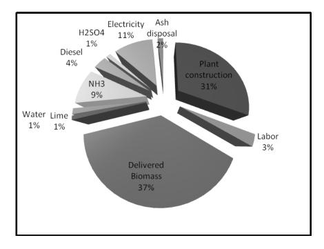
Figure 3. Ethanol unit production cost breakdown.
